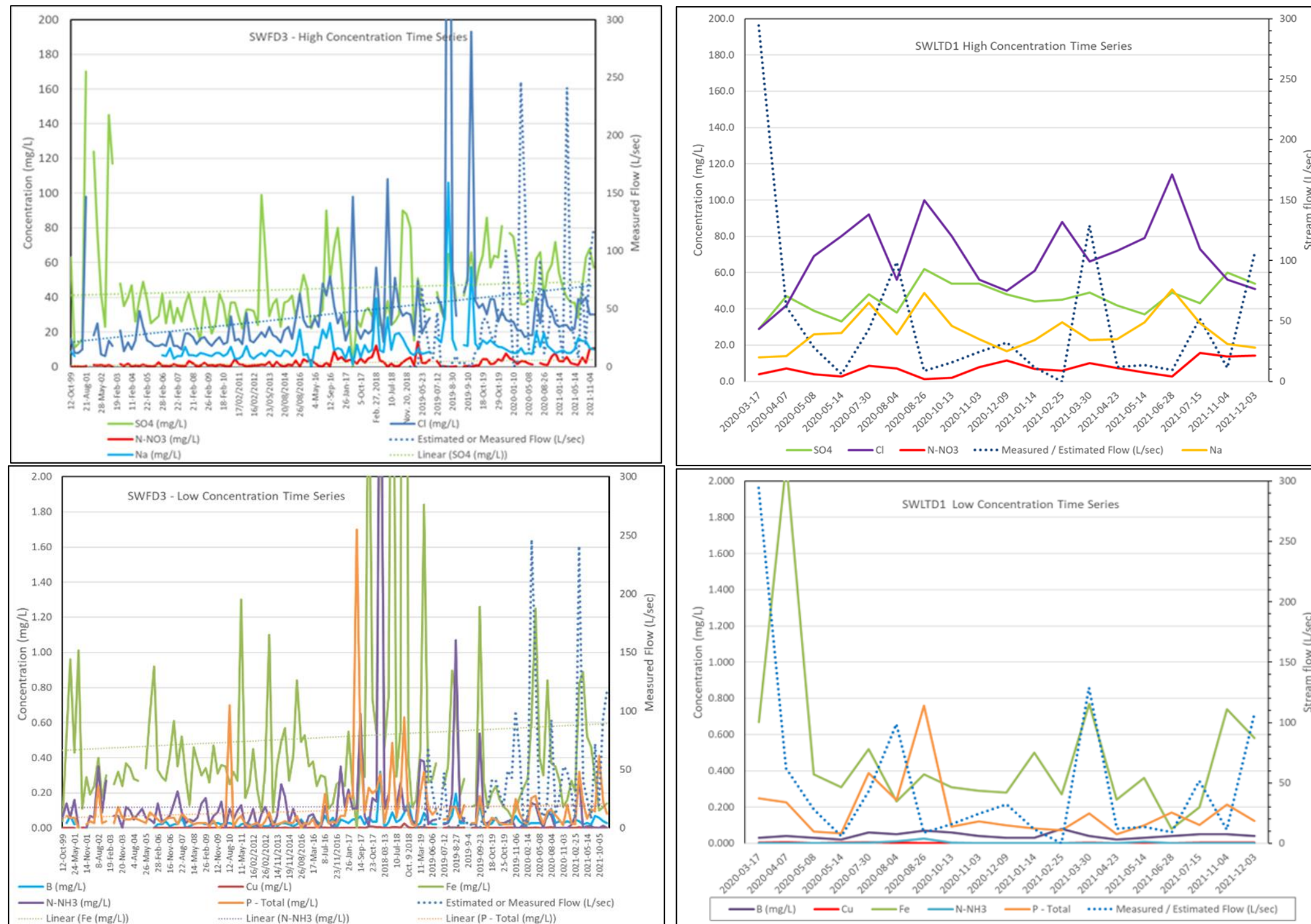
Figure 22 Time Series of Selected Water Quality Variables for SWFD3 and SWLTD1 (2020-03-17 to 2021-12-03) for “High Concentrations” (Cl, Na, NO 3 -N and SO 4 ) and “Low Concentrations” (Boron, Cu, Fe, NO 3 -N and P-total)
