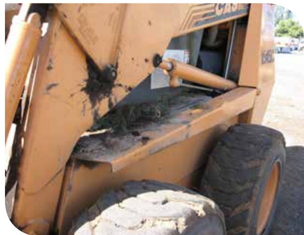
Plant material attached to bobcat.
