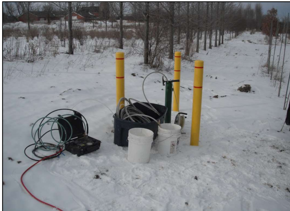
Photograph 2.2-8 Well development at completed piezometer
