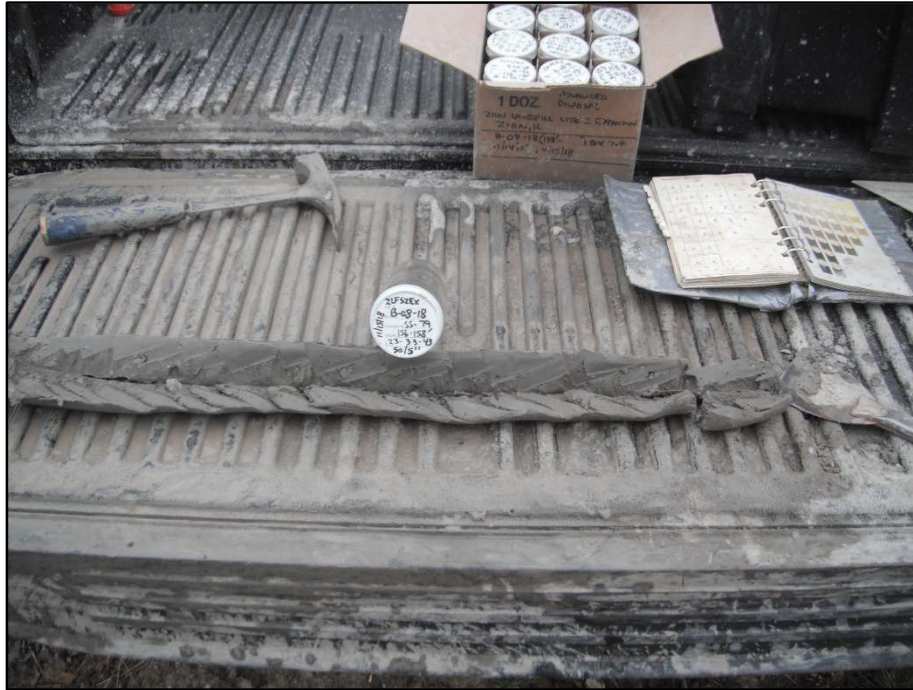
Photograph 2.2-11 Typical section of the Lower Till
