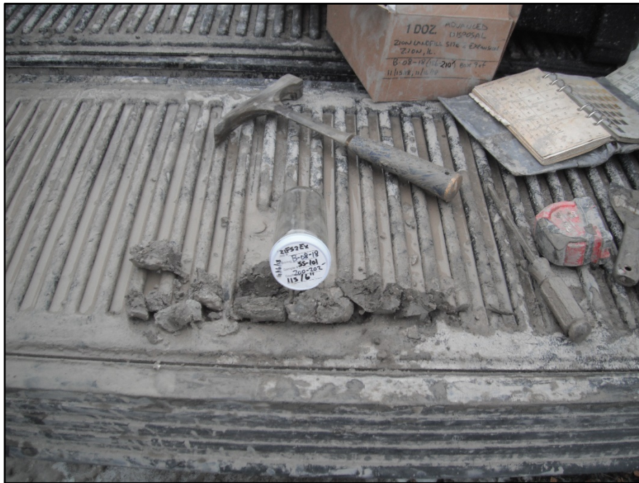
Photograph 2.2-12 Typical section of the Basal Drift
