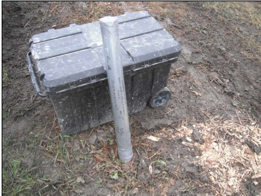
Photograph 2.2-3 Shelby tube used for collection of sample for geotechnical laboratory analysis
