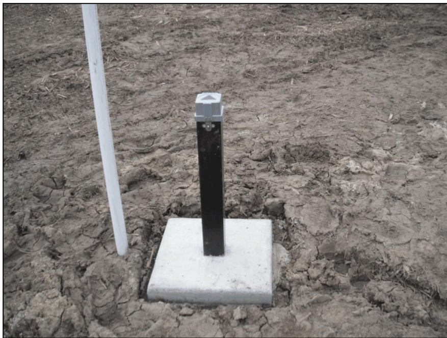
Photograph 2.8-1 Typical Monitoring Well
