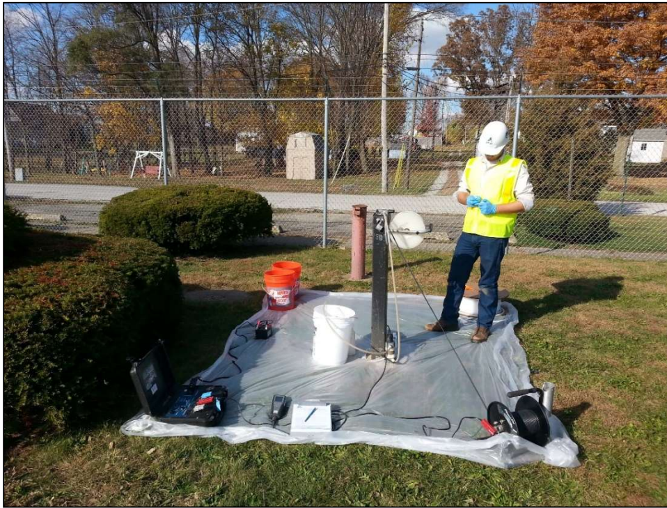
Photograph 2.8-2 Sampling of a typical monitoring well
