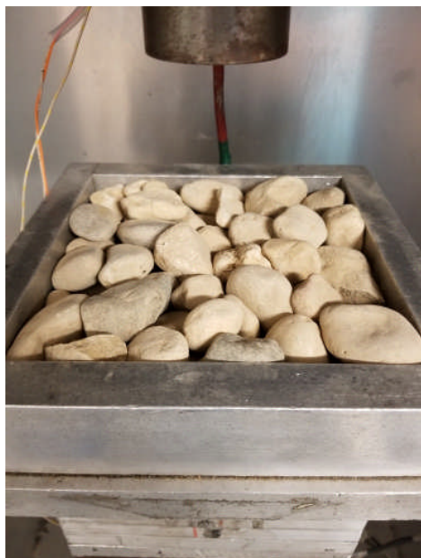
Leachate collection aggregate in SIM test box
