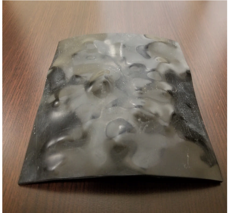
Geomembrane after SIM test
