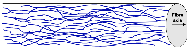
Fibre B: High-tenacity fibre - oriented molecular chains (crystalline regions)
