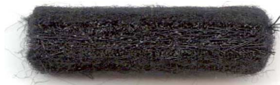
Fig. 3. Photograph of 3-layer structure geotextile.
