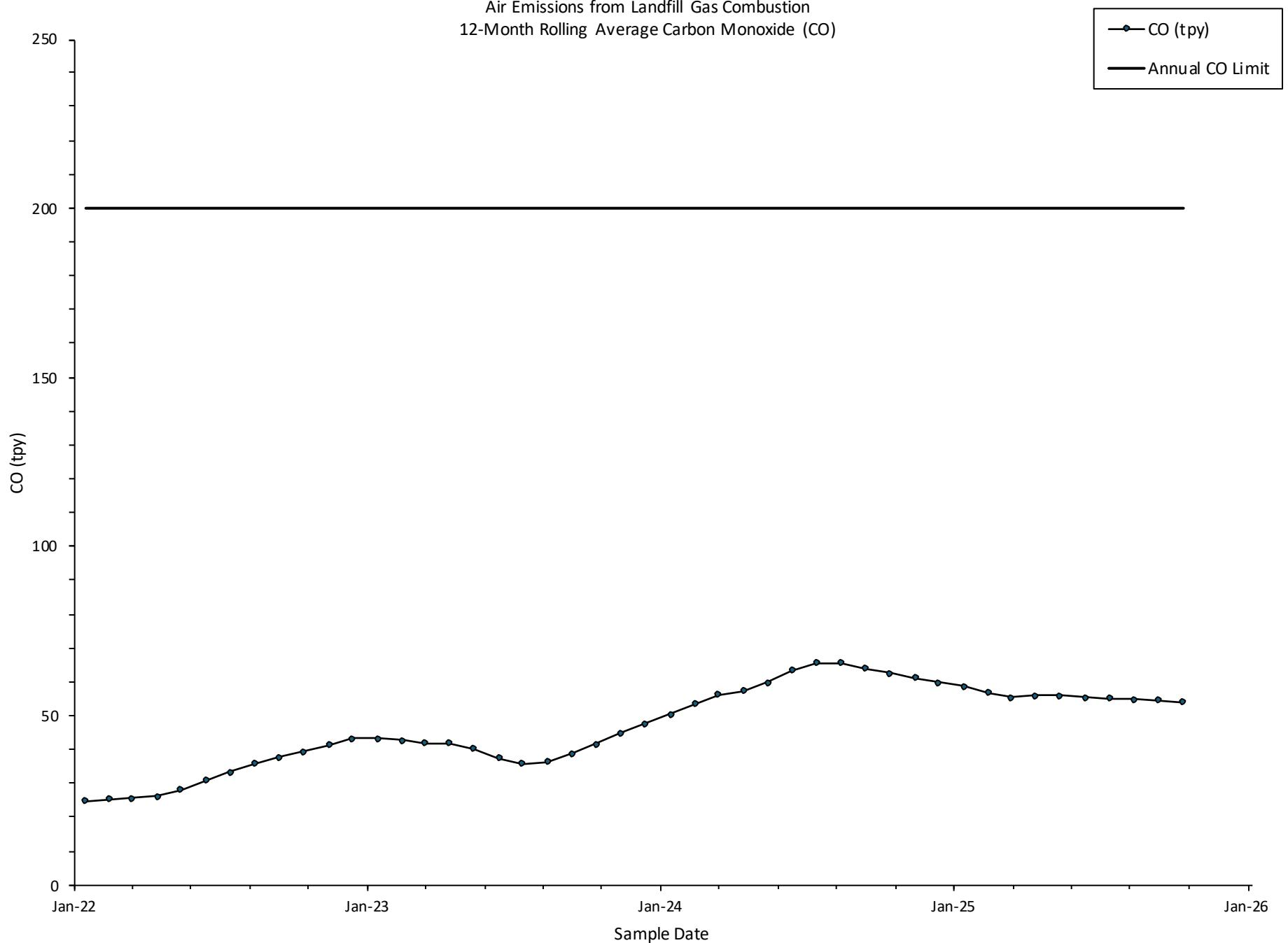
Air Emissions from Landfill Gas Combustion
